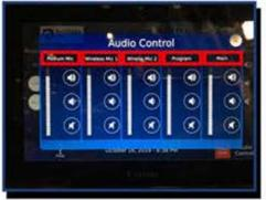
Podium Mic Wireless Mic 1 Wireless Mic 2 Program Main Volume Up, Down, & Mute. For projector use in Audio Only mode use controls for projector and use screen wall
