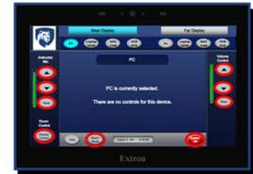
4. Room Controls: Instructor Mic & Volume Control Up, Down, Mute Display Control Room Mode
